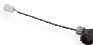
Ready-made cable Type FL33X33X 3 x 0,75 mm 2 with 3-pin bayonet connector 16 S 90° angle
